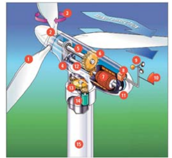
Main components of generation unit: 1-Blades; 2-Rotor; 3-Pitch; 4-Brake; 5-Low speed shaft; 6-Gearbox; 7-Generator; 8-Controller; 9-Anemometer; 10-Wind vane; 11-Nacelle; 12-High speed shaft; 13-Yaw drive; 14-Yaw motor; 15-Tower.
