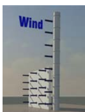
Fig. 2: Schematic view of the two structure examples for which static wind pressures were calculated according to both NBR and UBC norms. Left: flat wall. Right: cylinder with a diameter of 6 meters. Both structures were assumed to be located on an open flat field. No pressures resulting from dynamic effects have been considered.
