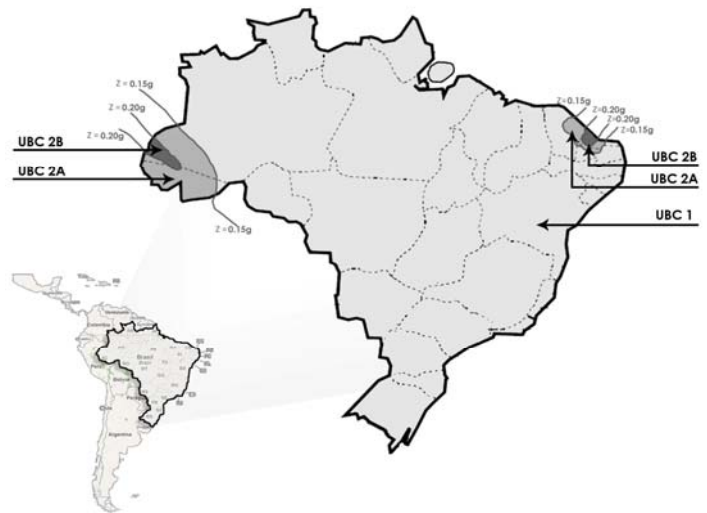
Fig. 4. Seismic Hazard Map of Brazil. Contour lines indicate the expected Maximum Horizontal Ground Acceleration Z, expressed in g ( 1g \approx 9.8 \text{ m/s}^2 ), according to an extrapolation from the Global Seismic Hazard Map, produced by the Global Seismic Assessment Program. Arrows indicate the classification of the different areas into UBC Zones according to the correspondance indicated in table 3.
