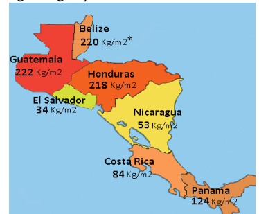
Fig. 3: Calculated wind pressures for same building at 10 m height at worst case conditions. (Value for Belize: extrapolated)
